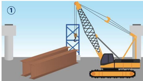
1. A large crane lifts the steel girder.
