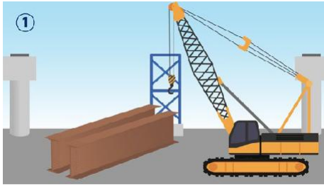
1. A large crane lifts the steel girder.
