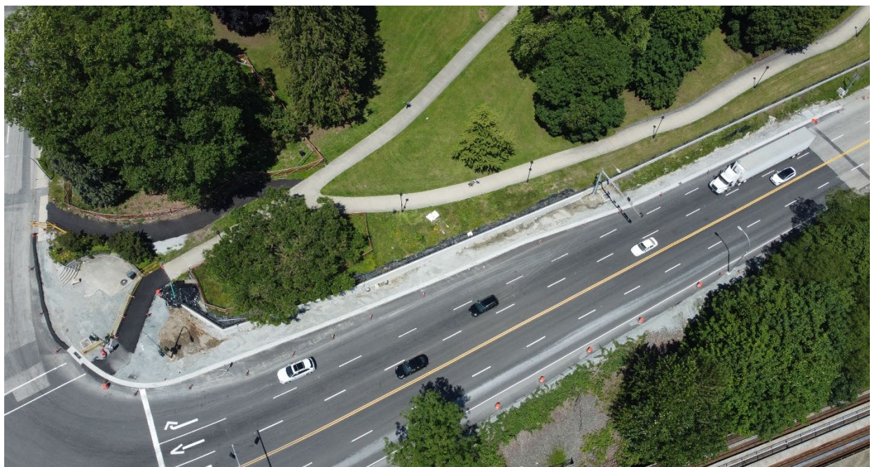
Figure 4 – Aerial of East Columbia Street near McBride Boulevard. The intersection has been elevated, widened, and repaved to its final configuration.
