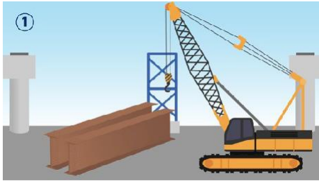
1. A large crane lifts the steel girder.
