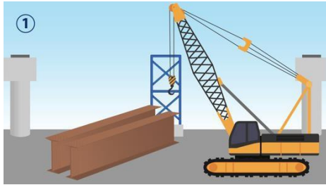
1. A large crane lifts the steel girder.
