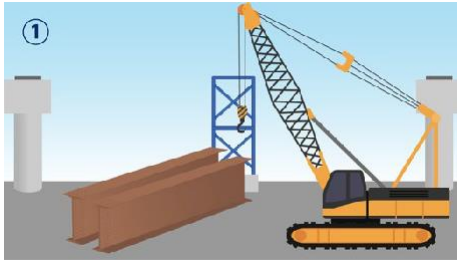
1. A large crane lifts the steel girder.
