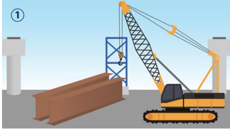
1. A large crane lifts the steel girder.
