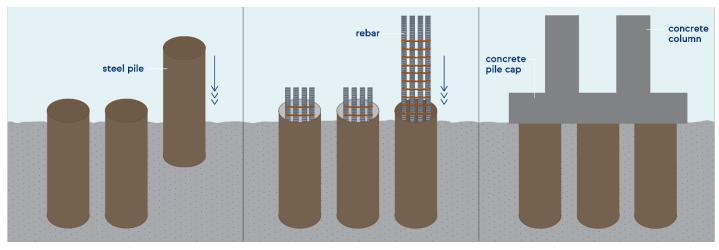
A pile cap is used on the S1 main tower foundation as well as piers N1, N3, S2 and S3. On pier N3, structural steel columns extend from bearing pedestals which sit directly on the pile cap.
