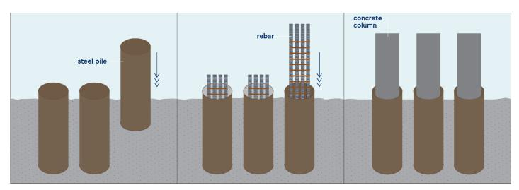
Concrete columns will be poured directly on top of the piles for piers N2, S4, S5, S6, S7, S8 and foundations for the Highway 17 off-ramp in Surrey.
