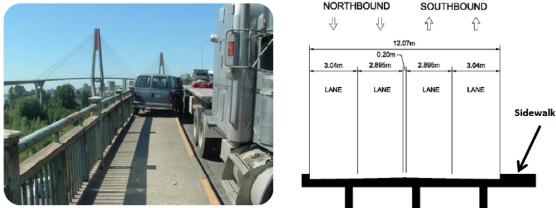
Figure 6: Sub-optimal Design Standards on the Existing Pattullo Bridge
